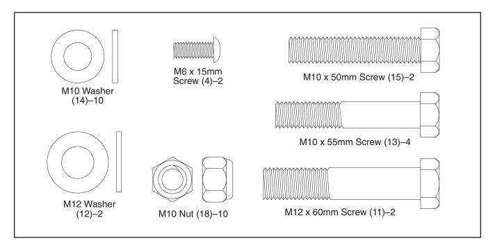
Attach the Base Crossbar (44) to the two Upright Bases (16) with two M10 x 50mm Screws (15) and two 10mm Washers (14) as shown.
